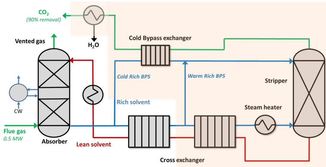
**Figure 1. Process Flow Diagram of the AFS Integrated 0.5-MW System at NCCC (Regeneration Equipment Supplied by URS in Peach)**
