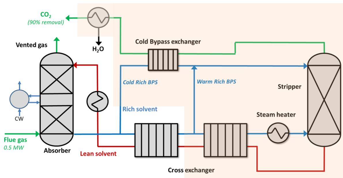
**Figure 2. Process Flow Diagram of the AFS Integrated 0.5-MW System at NCCC (Regeneration Equipment Supplied by URS in Peach)**
