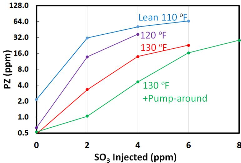
Figure 6. PZ Emissions Decreased with Increasing Lean Solvent Temp and with Pump-Around Water Wash Absorber Bed Operation
