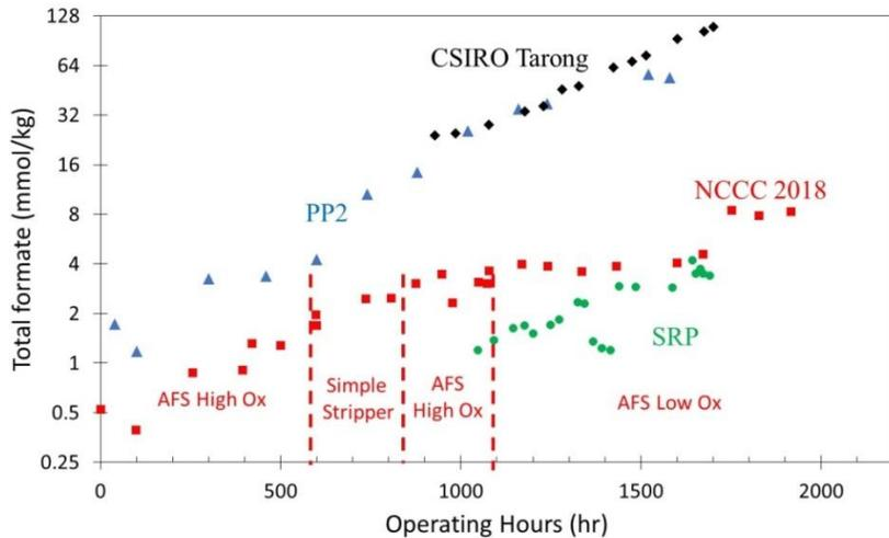
**Figure 5. Accumulation of Total Formate (Indicator of Thermal Degradation Products) in the PZ Solvent at NCCC and Other Campaigns**
