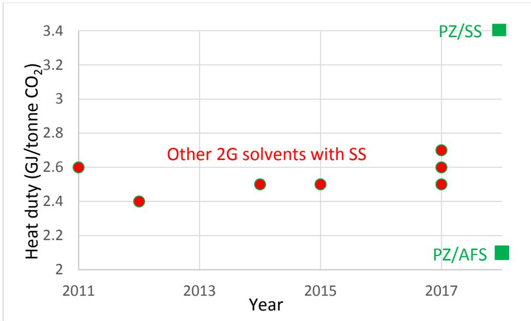
**Figure 10. Heat Duty of Second Generation Solvents Tested at NCCC (90% Capture; Not Corrected for Heat Loss)**
