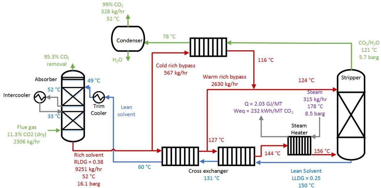
Figure 11. Optimal PZ/AFS Conditions as Determined by NCCC Testing
