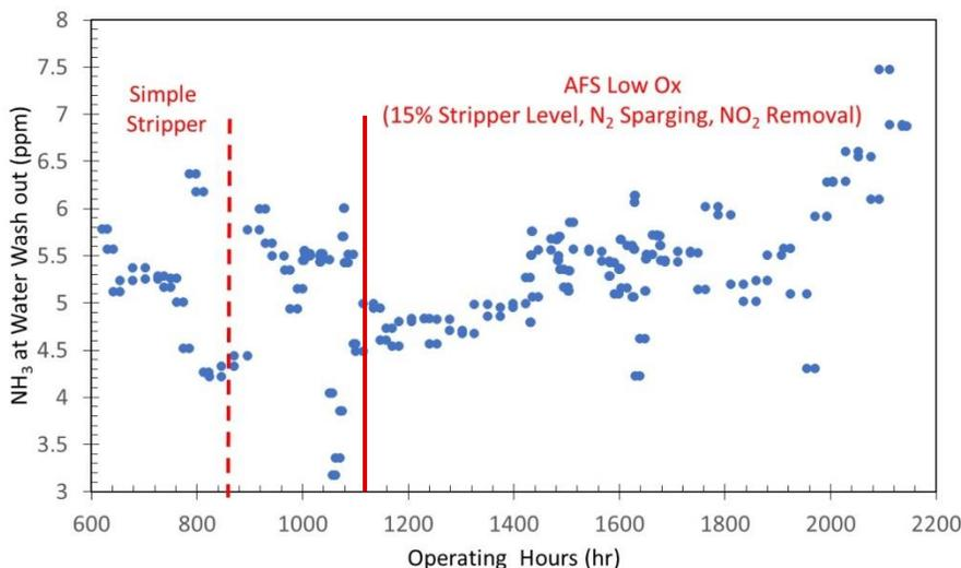
**Figure 4. Ammonia Emissions (Measured by FTIR; Indicator of Oxidation)**
