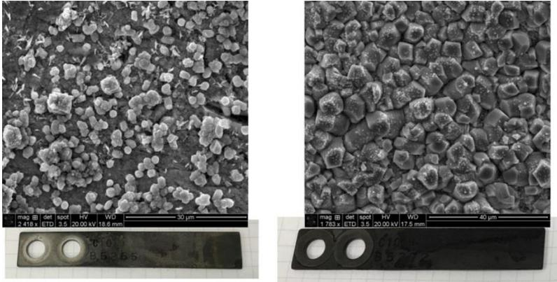
**Figure 9. Protective  $\text{FeCO}_3/\text{Fe}_3\text{O}_4$  Layer on Carbon Steel at 115 Hrs Exposure (Left - Cold Rich Bypass - Incomplete Layer; Right - AFS Sump - Protective Layer)**
