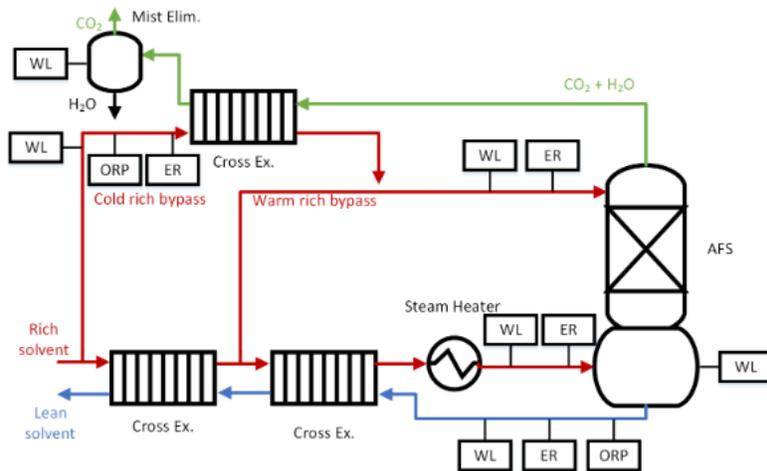
**Figure 8. PFD of AFS Corrosion Coupon Locations**
