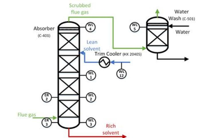
Figure 7. PFD of Absorber Corrosion Coupon (WL) and Electrical Resistance Corrosion Probe (ER) Locations
