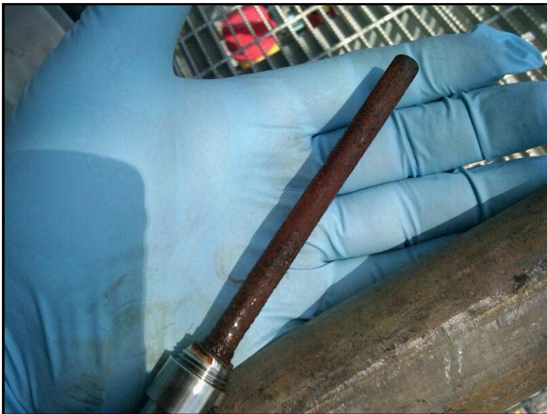
Figure 20: Typical ER Probe
