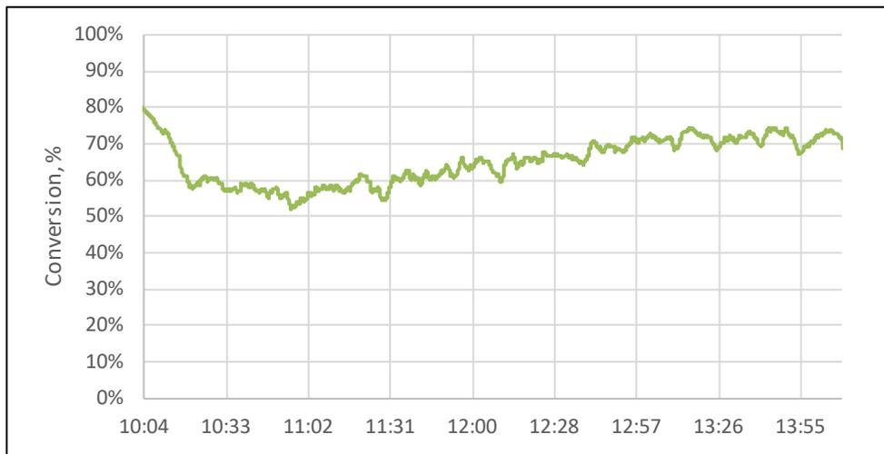
**Figure 18. Syngas Conversion in the SCL Reducer**
