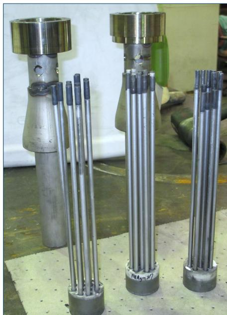
Figure 26. MPT Membrane Bundles and Housing Units
