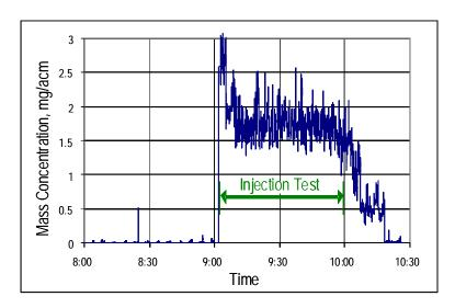
Figure 6-11. PPC Particulate Monitor Output during Solids Injection Test.
