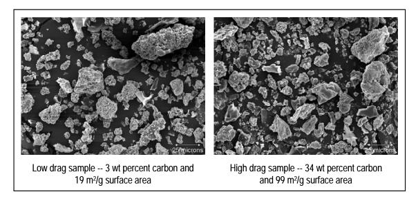
Figure 4-26. SEM Photographs of Low and High Drag Samples from Falkirk Lignite.
