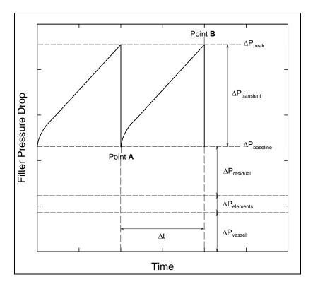
Figure 4-29. Graphical Illustration of Terms Used in PCD Sizing.
