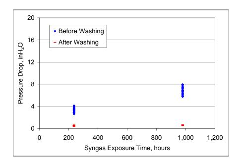
Figure 4-13. Pressure Drop versus Syngas Exposure Time for Fine Fiber Dynalloy Elements.
