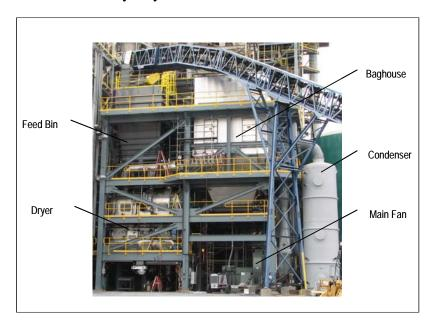
Figure 2-10. Fluid Bed Dryer System.
