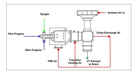
Figure 7-3. Flow Schematic of the Piloted Syngas Burner and Combustion Turbine.
