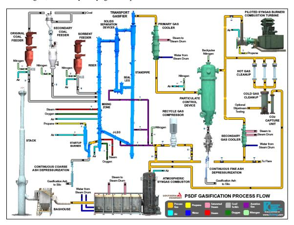
Figure 1-1. PSDF Gasification Process Flow Diagram.
