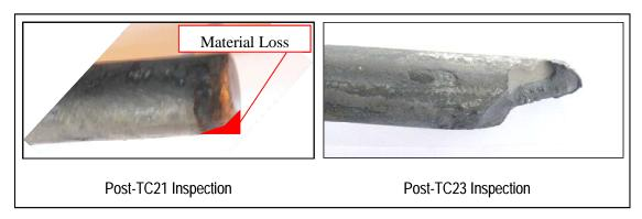
Figure 6-6. Post-TC21 and Post-TC23 Inspections of Worn HR-160 Thermowell.
