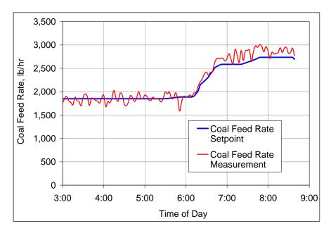
Figure 6-30. Coal Feed Rate Response to Setpoint Changes.
