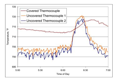
Figure 4-16. Filter Element Thermocouple Response during Bridging.
