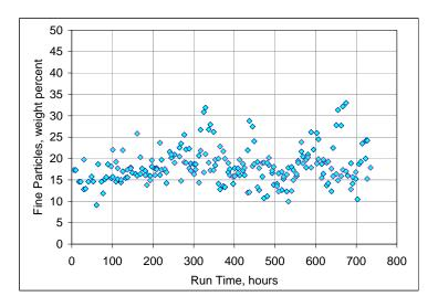
Figure 2-16. Percentage of Fine Particles in As-Fed Lignite.
