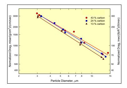
Figure 4-24. Lab-Measured Drag as a Function of Particle Size with PRB Subbituminous Coal Ash.
