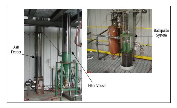
Figure 4-2. Cold Flow PCD Model.
