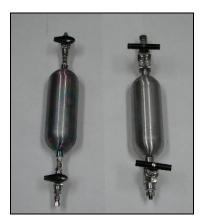
Figure 6-16. Bomb Sampler Cylinders.
