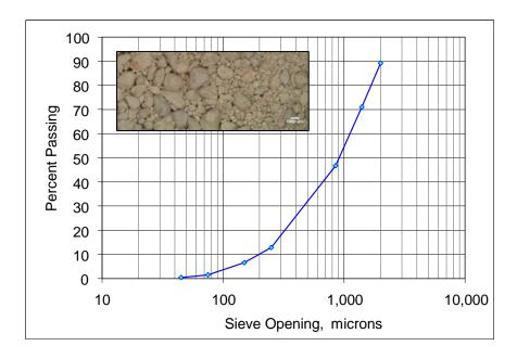
Figure 3-8. Kaolin Particle Size Distribution.
