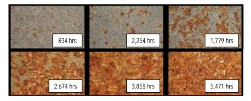
Figure 4-3. Micrographs of FEAL Filter Media Showing Progression of Iron Oxide Scale.
