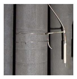
Figure 4-17. Filter Element Resistance Probe.
