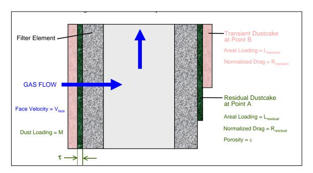
Figure 4-30. Dustcake Development at Points A and B in Figure 4-29.
