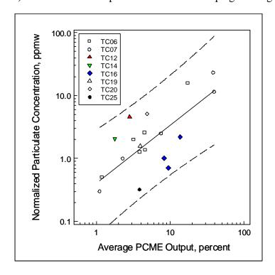
Figure 6-9. Comparison of PCME Particulate Monitor Response to Actual Mass Concentration.
