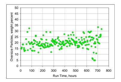
Figure 2-15. Percentage of Oversize Particles in As-Fed Lignite.
