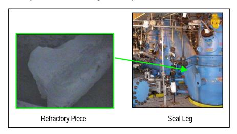
Figure 3-7. Gasifier Seal Leg Obstruction.
