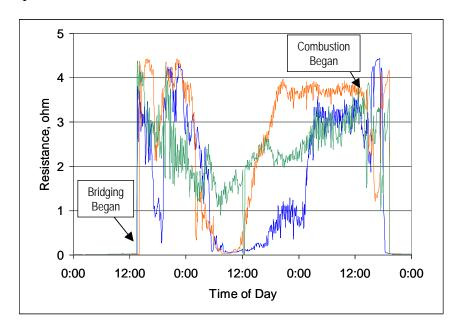
Figure 4-20. Resistance Probe Response during On-Line Bridging Removal.
