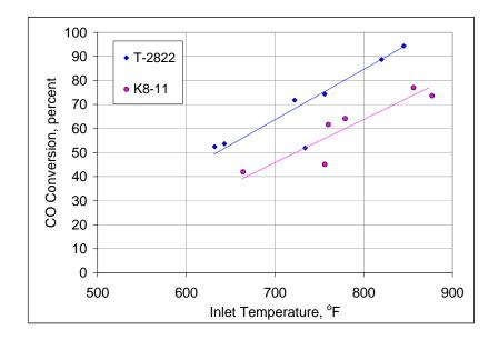
Figure 5-3. T-2822 and Katalco K8-11 Shift Catalyst Performance Comparison.
