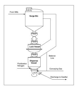
Figure 2-18. Original Coal Feed System.
