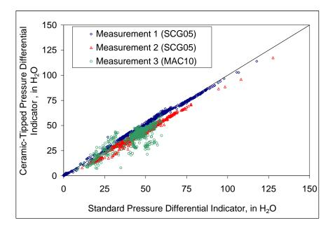
Figure 6-4. Measurements of Ceramic-Tipped Pressure Differential Indicators Compared to Standard Pressure Differential Indicators.
