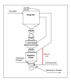
Figure 2-21. Original Coal Feeder Balance Line Location.
