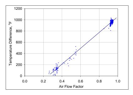
Figure 3-13. Temperature Difference as a Function of Air Flow to LMZ.
