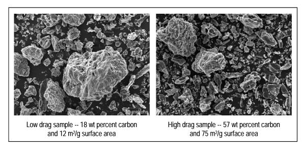
Figure 4-28. SEM Photographs of Low and High Drag Samples from Freedom Lignite.
