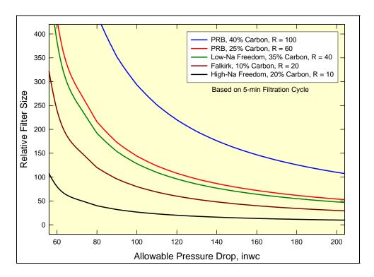
Figure 4-31. Effect of Transient Drag on Required PCD Size at a Given Allowable Pressure Drop.
