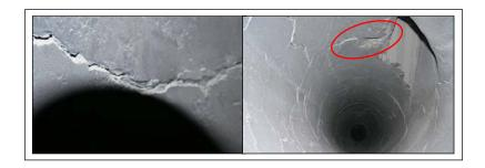
Figure 3-4. Inspection of Actchem 85VC Refractory following Initial Operation.
