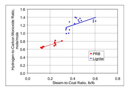
Figure 3-17. Syngas Hydrogen-to-Carbon Monoxide Ratio versus Steam-to-Coal Ratio.
