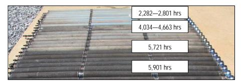
Figure 4-4. Cleaned FEAL Elements Arranged by Exposure Time.
