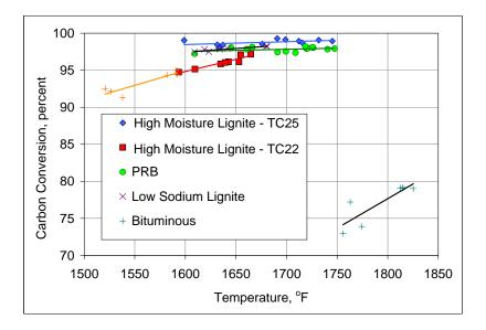
Figure 3-9. Carbon Conversion as a Function of Gasifier Outlet Temperature.
