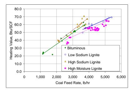
Figure 3-11. Syngas Heating Value as a Function of Coal Feed Rate.
