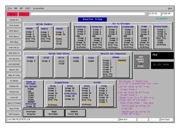
Figure 6-33. DCS Safety Interlock System.
