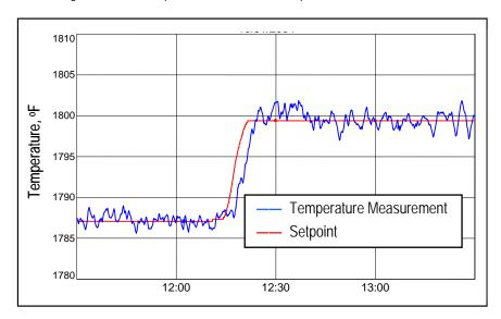
Figure 6-29. Gasifier Temperature Response to Setpoint Change using Pseudo-Fuzzy Control Plane.
