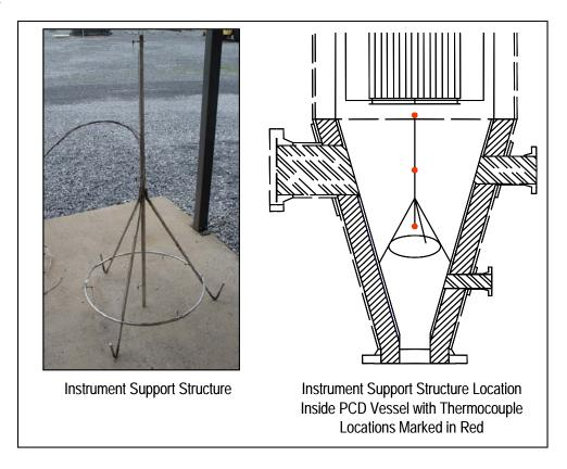
Figure 4-19. PCD Hopper Thermocouple Support Structure.
