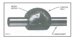
Figure 2-19. Vent Valve Replacement on Original Coal Feeder.
