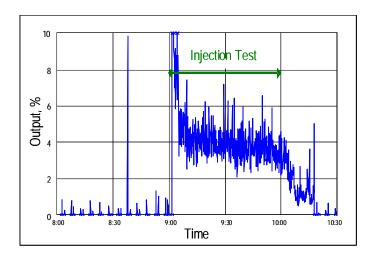
Figure 6-8. PCME Particulate Monitor Output during Solids Injection Test.
