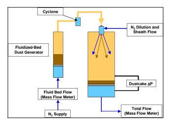
Figure 4-22. Laboratory Apparatus for Measuring Drag of Re-suspended Gasification Ash.
