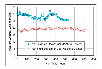
Figure 2-17. Moisture Content of As-Fed Lignite before and after Fluid Bed Dryer Installation.
