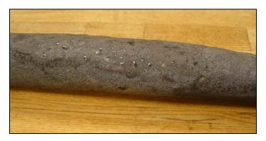
Figure 4-14. Section of Damaged Titanium Filter Element.
