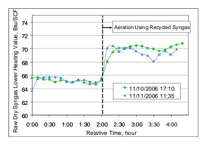
Figure 3-15. Effect of Recycle Gas Use for Gasifier Aeration on Syngas Heating Value.
