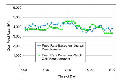
Figure 6-2. Coal Feed Rate Measurements.
