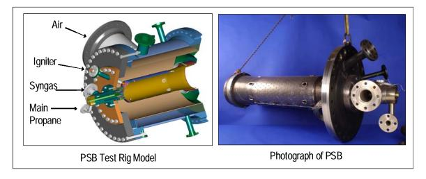
Figure 7-4. Piloted Syngas Burner Model and Photograph.
