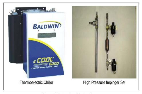
Figure 6-27. Gas Conditioning System.
