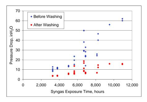
Figure 4-9. Pressure Drop versus Syngas Exposure Time for Pall PSS FEAL Elements.
