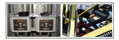
Figure 2-6. Microwave Solids Flow Switches.
