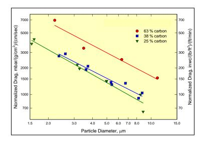
Figure 4-25. Lab-Measured Drag as a Function of Particle Size with High-Sodium Freedom Lignite Ash.
