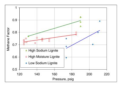
Figure 3-12. Syngas Methane Content as a Function of Pressure.
