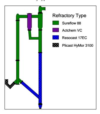
Figure 3-2. Gasifier Refractory Layout.
