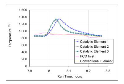
Figure 5-6. Catalytic Filter Element Temperatures during Thermal Upset at Hour 8.
