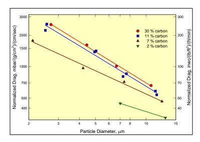
Figure 4-23. Lab-Measured Drag as a Function of Particle Size with Falkirk Lignite Ash.
