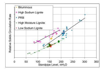
Figure 3-10. Solids Circulation Rate as a Function of Standpipe Level.
