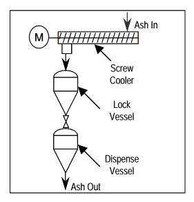
Figure 7-5. Schematic of Original Ash Cooling and Depressurization Systems.
