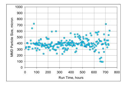
Figure 2-14. Particle Sizes of As-Fed Lignite.
