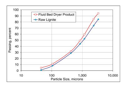
Figure 2-11. Particle Size Distributions of Lignite Processed in Fluid Bed Dryer and of Raw Lignite.
