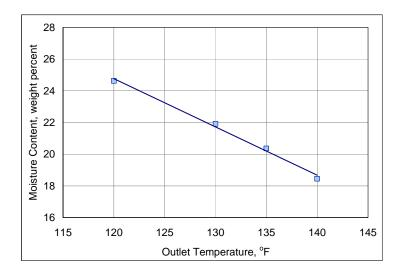
Figure 2-12. Product Moisture Content versus Fluid Bed Dryer Outlet Temperature.
