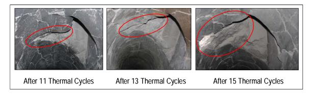
Figure 3-6. Refractory Loss at the Inlet of the First Solids Separation Device.
