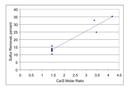
Figure 3-16. Sulfur Removal as a Function of Calcium-to-Sulfur Molar Ratio.
