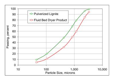
Figure 2-13. Particle Size Distributions of Pulverized Lignite and of Lignite Processed in Fluid Bed Dryer.
