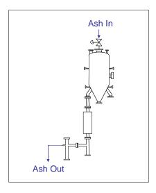
Figure 7-6. CFAD Schematic.
