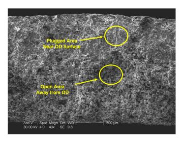
Figure 4-7. Photomicrograph of Plugged and Open Areas of FEAL Element.
