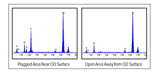
Figure 4-8. EDX Spectra from Plugged and Open Areas Indicated in Figure 4-7.
