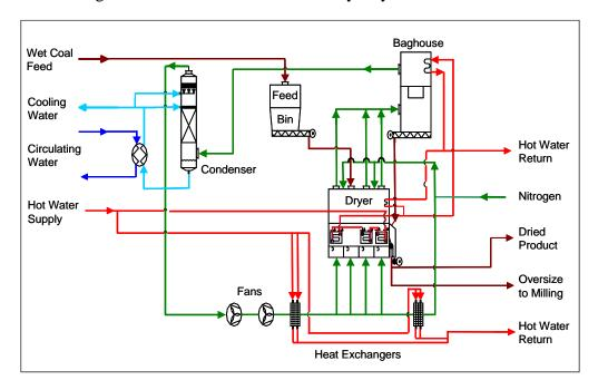
Figure 2-9. Fluid Bed Dryer System Flow Diagram.
