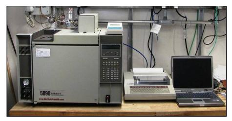
Figure 6-21. On-Line Laboratory GC Unit for PCD Inlet Gas Analysis.
