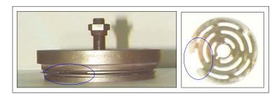
Figure 7-1. Valve Failure on Original Recycle Gas Compressor
