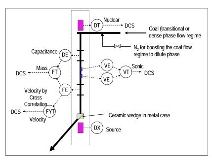
Figure 6-1. Schematic of Nuclear Densitometer Layout for Developmental Coal Feed System.
