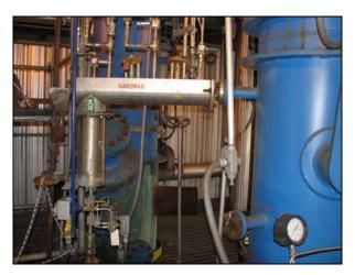
Figure 6-14. Gasifier Solids Sampling System.
