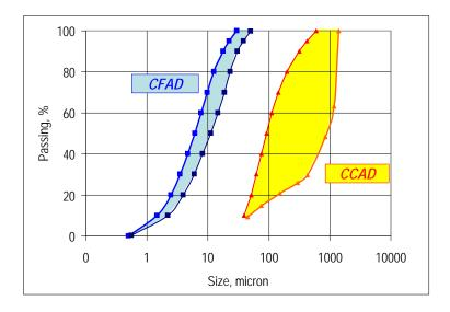
Figure 7-7. Particle Size Distributions of Gasification Ash Processed by the CFAD and CCAD Systems.
