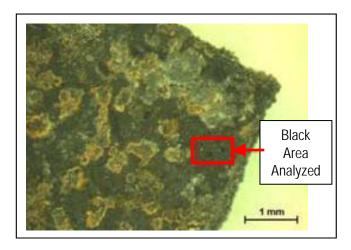
Figure 4-5. Photomicrograph of FEAL Filter Element Section Showing Pitted Areas with Iron Oxide Borders.
