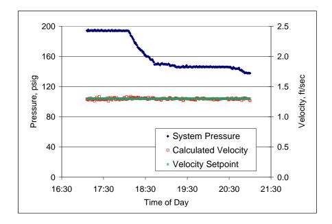
Figure 6-32. Gasifier J-Leg Velocity Control Response to Pressure Change.
