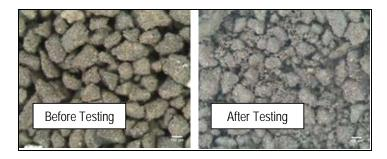
Figure 5-5. Photomicrographs of Johnson Matthey Katalco K8-11 Shift Catalyst before and after Testing.
