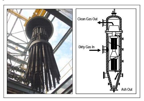
Figure 4-1. Siemens Particulate Control Device.
