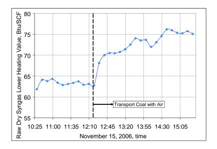
Figure 3-14. Effect of Transport Air on Syngas Lower Heating Value.
