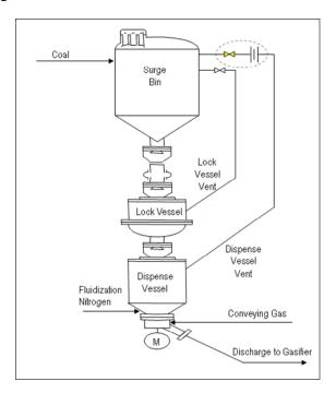
Figure 2-20. Original Coal Feeder Vent Valve Location.
