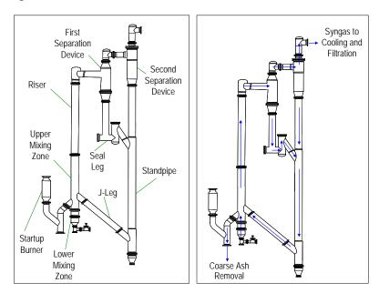
Figure 3-1. Schematic of Transport Gasifier.
