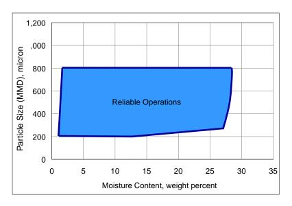
Figure 2-22. Original Coal Feeder Operating Envelope.
