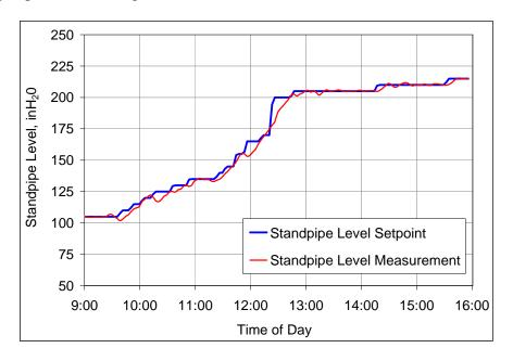
Figure 6-31. Standpipe Level Response to Setpoint Changes.
