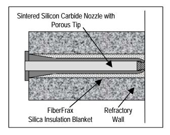
Figure 6-3. Schematic of Ceramic Tip for Pressure Differential Indicator.
