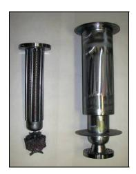
Figure 6-19. Disassembled Reflux Probe.
