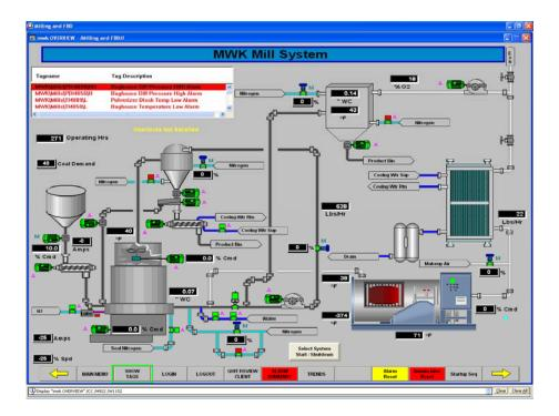
Figure 2-8. Mill System Human Machine Interface.
