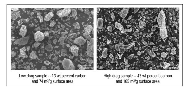
Figure 4-27. SEM Photographs of Low and High Drag Samples from PRB Coal.
