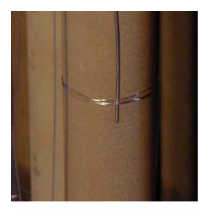
Figure 4-15. Filter Element Thermocouple.
