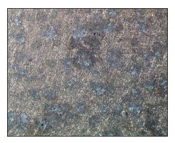
Figure 4-11. Fine Fiber HR-160 Filter Media with 979 Syngas Exposure Hours.
