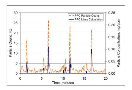
Figure 6-10. PPC Particulate Monitor Output during Low Particulate Loading.
