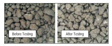
Figure 5-4. Photomicrographs of Sud-Chemie T-2822 Shift Catalyst before and after Testing.
