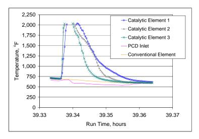
Figure 5-7. Catalytic Filter Element Temperatures during Thermal Upset at Hour 39.
