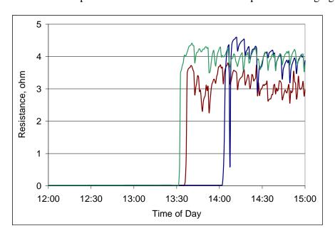
Figure 4-18. Filter Element Resistance Probe Response during Bridging.
