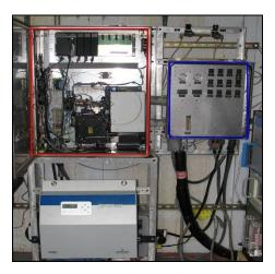
Figure 6-24. FTIR Gas Analysis System.
