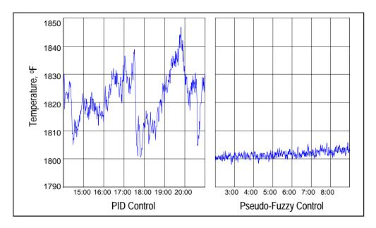
Figure 6-28. Comparison of Gasifier Temperature Control Schemes.
