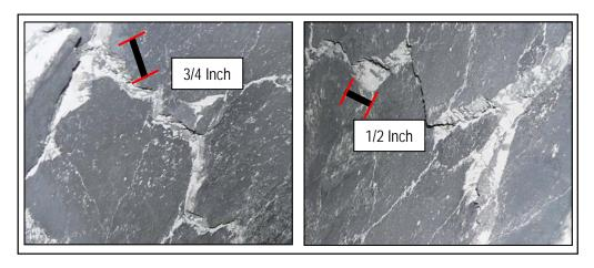
Figure 3-5. Cracking of Actchem 85VC Refractory after Eleven Thermal Cycles.
