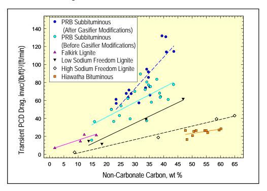
Figure 4-21. PCD Transient Drag versus Carbon Content of In-Situ Samples.
