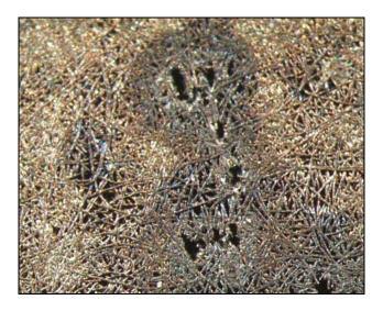
Figure 4-10. Coarse Fiber Dynalloy HR-160 Filter Media with 2,698 Syngas Exposure Hours.
