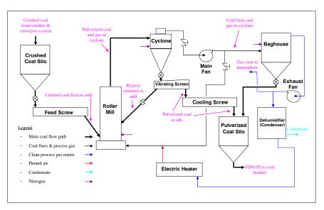
Figure 2-1. Coal Preparation Process Flow Diagram
