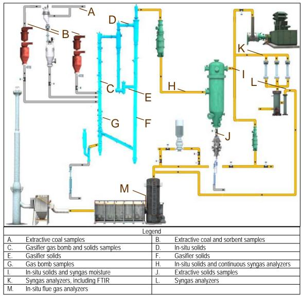
Figure 6-12. Sampling Locations of the PSDF Gasification Process.
