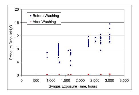
Figure 4-12. Pressure Drop versus Syngas Exposure Time for Coarse Fiber Dynalloy Elements.
