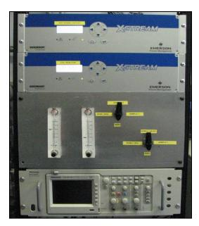
Figure 6-25. CO<sub>2</sub> Capture and Water-Gas Shift Reaction Analyzers.
