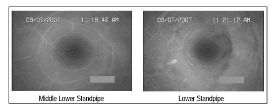
Figure 3-3. Lower Standpipe Refractory after 70 Thermal Cycles.
