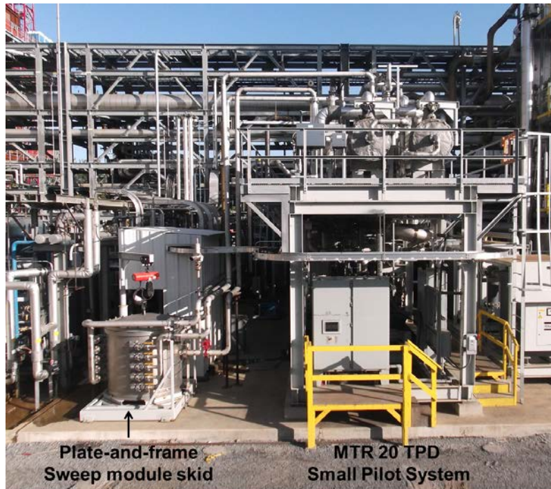
Figure 3. Picture showing the plate-and-frame sweep skid next to the larger MTR 20 TPD small pilot unit at NCCC.
