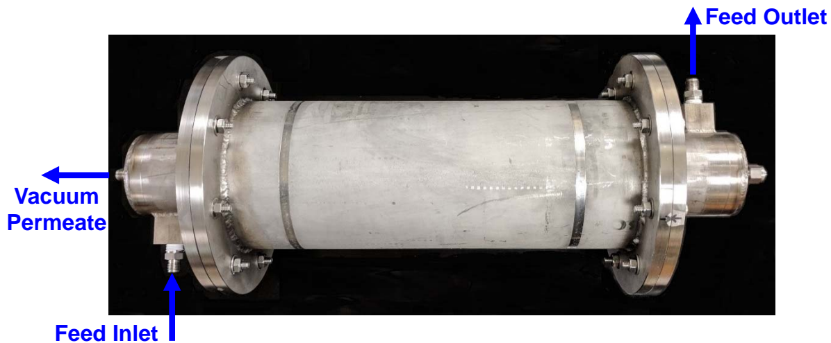
Figure 2. Spiral-wound membrane module consisting of the membrane element inside a housing.
