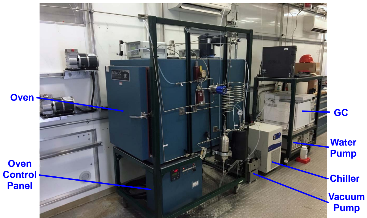
Figure 4. The setup of the gas permeation unit at NCCC (photo credit: Tony Wu, NCCC).
