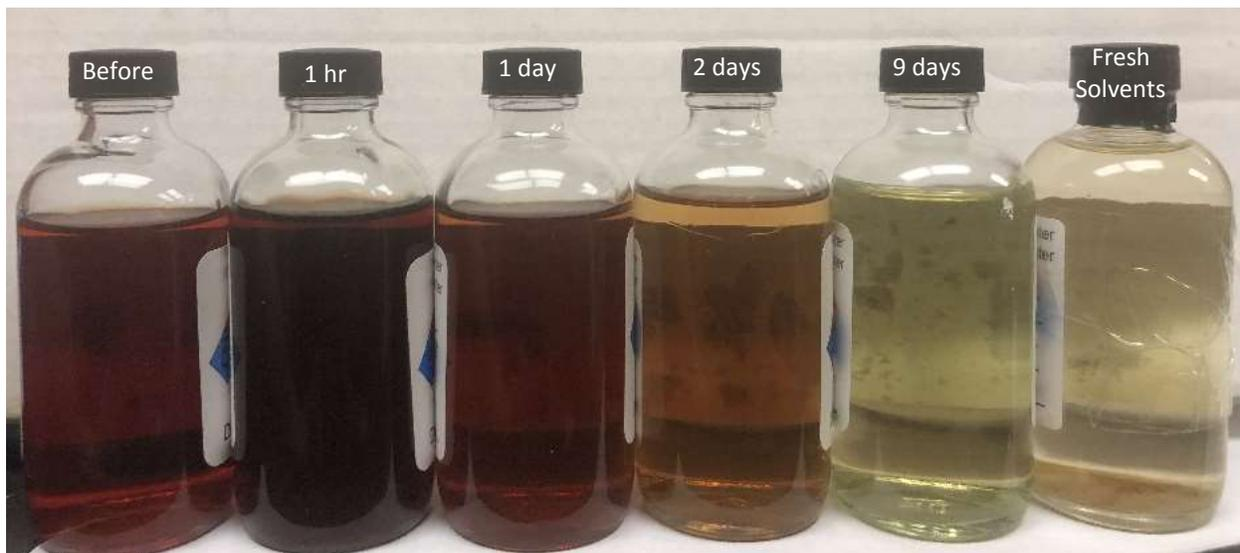
**Figure 3. Visual Effects of Solvent by Carbon Bed**
