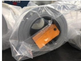
Figure 2: Left, an example design of sorption/desorption module with Microlith coil around an axial-flow gas distribution system (other options include planar arrangement with flow-through). Right, Microlith coils coated with sorbent holding approximately 200 sq ft of coated mesh.
