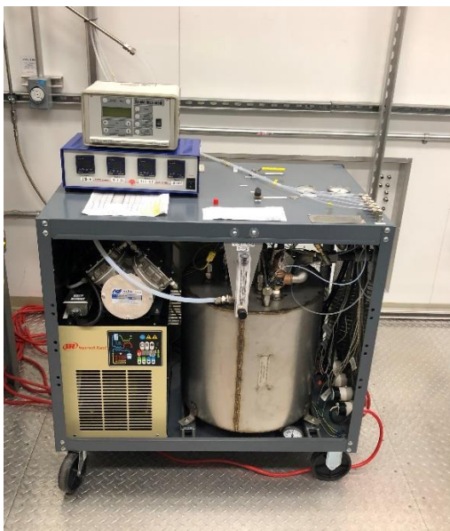
Figure 6: PCI test skid installed on the flue gas flow stream at the National Carbon Capture Center.
