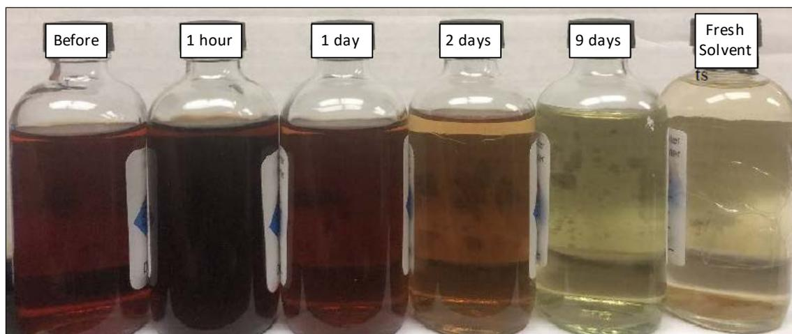
**Figure 13. Piperazine Solvent Color Changes with the Use of Carbon Filters Over a Nine-Day Period**
