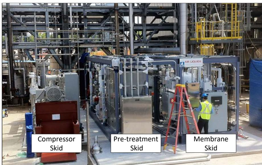
Figure 18. Air Liquide Cold Membrane Process Skids
