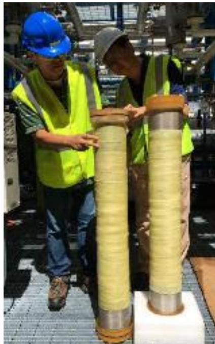
**Figure 7.** Photograph of 8-inch diameter membrane cartridges.
