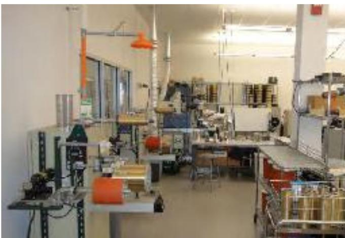
**Figure 2.** PEEK hollow fiber extrusion lines.
