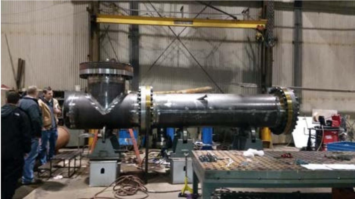
Figure 9. Picture of hydrotesting of burner chamber shell at Gaspar, Inc.
