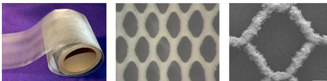
Figure 1: Microlith mesh coated with sorbent – cell opening 600 \mu\text{m} .
